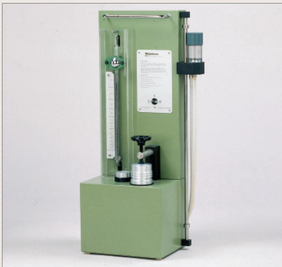
Air pycnometer according to Langer
