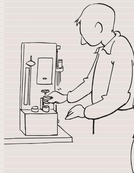
As soon as the under pressure is stable the value can be read and the levelling vessel is placed in the upper position.
