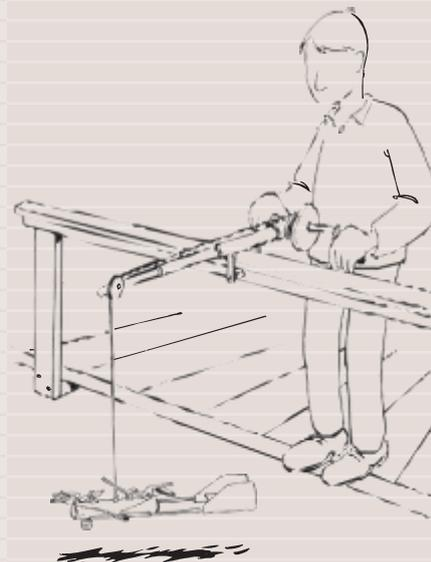
**The sealing valves of the watertrap are opened before the sampler is lowered (spring operated).**
