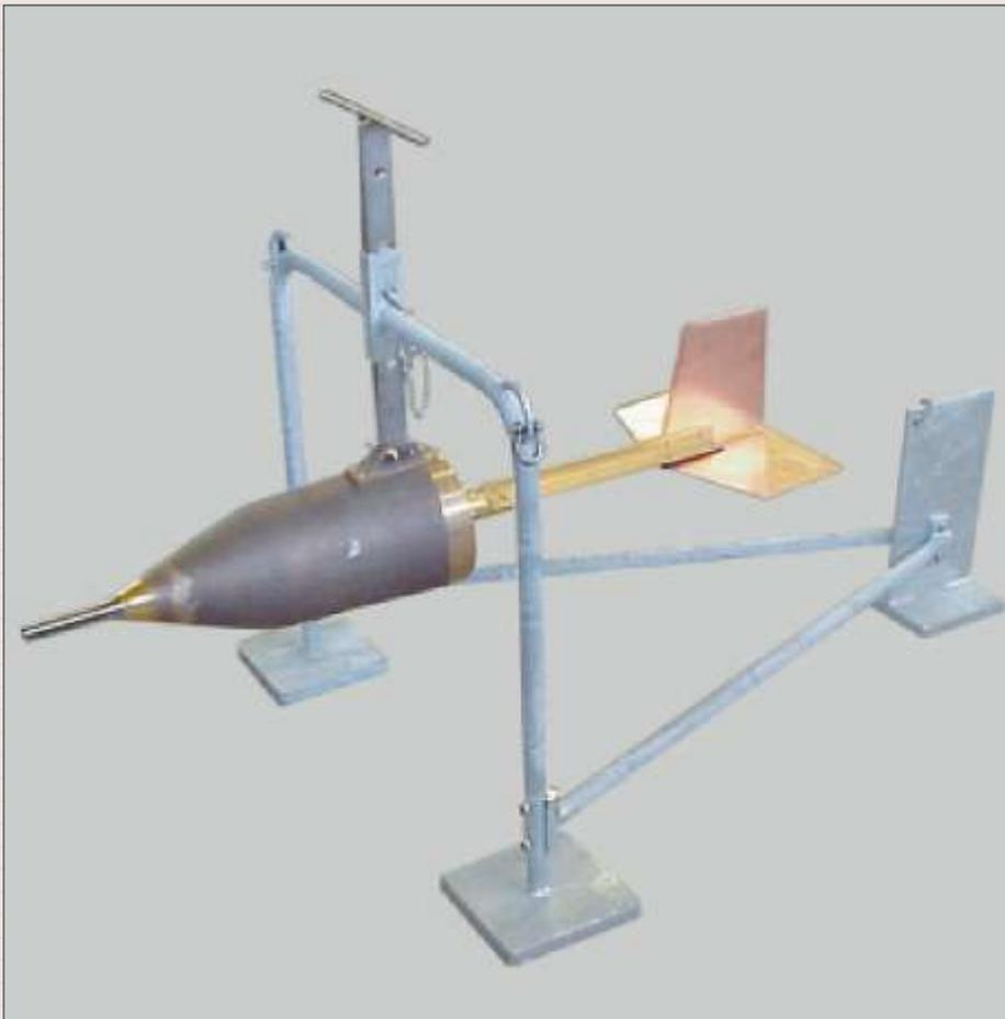
Suspended load sampler Delft bottle type
